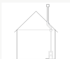
5. Flat ceiling with roof space and offset
